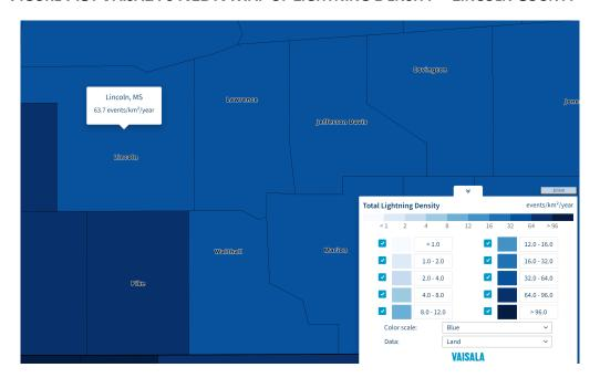
FIGURE F.5: VAISALA'S NLDN MAP OF LIGHTNING DENSITY - LINCOLN COUNTY<sup>37</sup>
